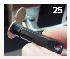
A view of the key and keyway (photo 26), confirms the striking resemblance to a Mul-T-Lock key and cylinder. Insert the key until it stops (photo 27). The key is tip stopped, so don't expect the key shoulders to contact the face of the cylinder plug. Rotate the key counterclockwise one quarter
