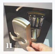
to the battery pack. The plug end of the cable looks like it should connect to a 9 volt battery, but it connects to the battery pack which uses four AA batteries. I used rechargeable batteries for demonstration purposes, but you should use alkaline batteries for longer life and less frequent battery changing.
