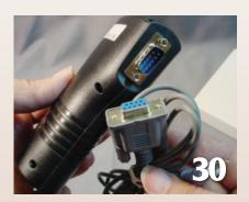
to both upload data from the lock and later download the data to your computer to identify when the lock was used and who was using it. The cable with a pin type jack is attached to the unit (photo
