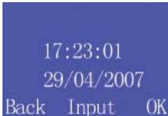
**Step 3:** Use the Navigation Buttons to adjust the date and time. When finished adjusting, highlight Input and press Ok.
