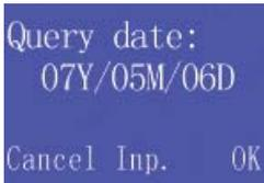
**Step 5:** Use the Navigation Buttons to adjust the date. When finished adjusting, highlight Inp. and press Ok.
