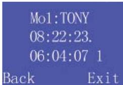
**Step 9:** Use the Navigation Buttons to view each matching record. Press Exit when finished.
