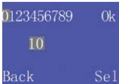
**Step 7:** Highlight the desired number and press Sel to select the number. Finally, highlight OK and press Sel to confirm.
