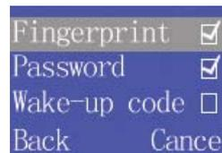
**Step 4:** Use the Navigation Buttons to highlight the desired Access Modes. Press Ok or Cancel to toggle the selection. Note: Fingerprint must be unchecked before enabling the Wake-up Code mode.
