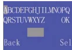
**Step 6:** Highlight the desired letters and press Sel to select the letter. Finally, highlight OK and press Sel to confirm.
