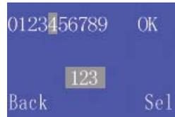
**Step 6:** Determine the number of records to view. Highlight the number you would like and press Sel. When finished, highlight Ok and press Sel.
