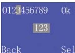
**Step 7:** Highlight the number you would like to add to the password and press Sel. When finished, highlight Ok and press Sel.
