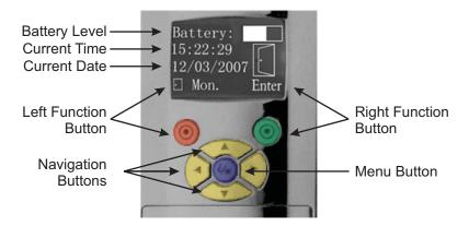
**Battery Level** - The battery level indicator represents the approximate percentage of battery use left in the current set up batteries.
