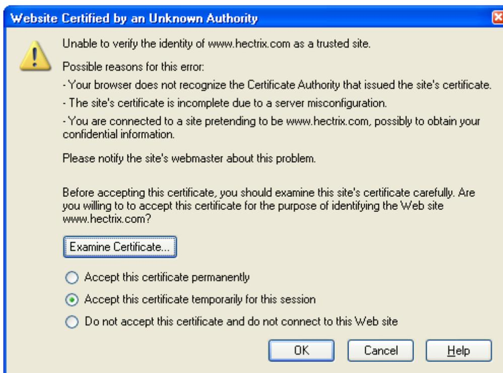
After selecting “Secure” login, the above screen will be displayed and to go on to login to view the web interface of ACTAtek External IP Smartcard Reader, select either “Accept this certificate permanently” or “Accept this certificate temporarily for this session”. It is recommended to have the temporarily selected if you are not using your PC / laptop for this http session, so that others cannot use this site without the proper authentication. Make the selection and click “OK”.
