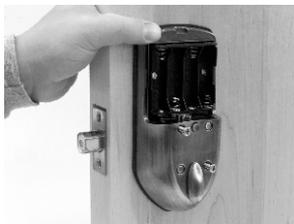
Locate the Bolt Direction Switch (A) just under the batteries. Make sure the Bolt Direction Switch corresponds with the direction that the bolt extends (B). In the example to the right, the bolt extends out of the left side of the door. Therefore the switch should be moved to the left as shown by the diagram (C).
