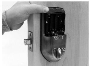
Locate the Bolt Direction Switch (A) just under the batteries. Make sure the Bolt Direction Switch corresponds with the direction that the bolt extends (B). In the example to the right, the bolt extends out of the left side of the door. Therefore the switch should be moved to the left as shown by the diagram (C).
