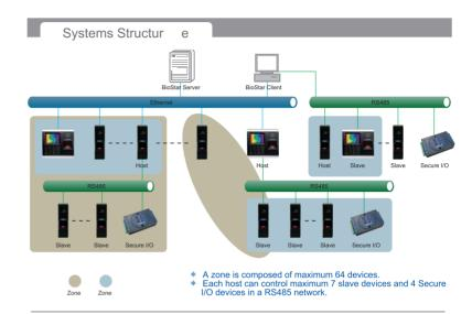
Compared to conventional access control systems, BioStar provides efficiency and stability by distributing intelligence to each door.
