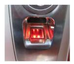
3) After the fingerprint sensor powers on, rest the enrolled fingerprint associated to the User ID on the sensor window to verify.
