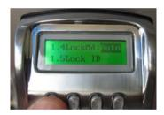
3) Message "Lock Mode Saved" will display and there will be an audible buzz of the solenoid engaging (if TUM is chosen) or disengaging (if Auto is chosen).
