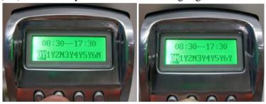
• If "Y" (Yes) is chosen for a specific day of the week, then the Specific User ID will have access to unlock the BioAxxis<sup>®</sup> ThumbLock<sup>®</sup> with their enrolled fingerprints and/or PIN Code, on that day of the week, during the **Date Range** and **Time Frame** that has already been set up. Once the Date Range or Time Frame has expired, the fingerprints and PIN Code associated to the Specific User ID will not be able to unlock the BioAxxis<sup>®</sup> ThumbLock<sup>®</sup>.
