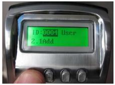
• Again, User IDs 1 thru 3 are Administrator (Master) Users that will have access at any time to unlock the door or program the BioAxxis<sup>®</sup> ThumbLock<sup>®</sup>. Users 4 thru 1000 are General Users that have access to unlock the door at times set up by one of the Administrator Users and have no programming rights to the BioAxxis<sup>®</sup> ThumbLock<sup>®</sup>.
