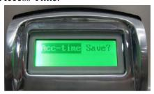
NOTE: The Time Setting chosen/created for the lock will override any specific Timed Access assigned for a specific User. For example, if ACC-TIME is chosen for the lock and set to Mon, Wed and Fri 9am to 5pm, Users will only have access to unlock the door during the set days and times, no matter what individual timed access was set for them. However, Administrators (User ID 1-3) will always have access to unlock the BioAxxis<sup>®</sup> ThumbLock<sup>®</sup>.
