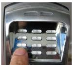
2) If PIN Code verification was successful, a single short beep will be heard, the green LED will flash and the BioAxxis<sup>®</sup> ThumbLock<sup>®</sup> will unlock (and remain unlocked for approximately four seconds).
