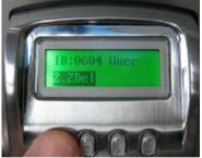
• "Del?" message will display. Press "M" to complete deletion of fingerprints associated to the specific User ID.
