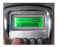
4) "PIN: CIPIN" will display, indicating that all PIN Codes have been deleted.
