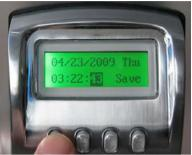
12) Choose the correct day of the week by using the Up/Down arrows until desired day of the week is chosen and press "M" to save selection.
