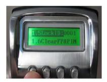
2) Use the up and down arrows to scroll to the desired lock ID <u>OR</u> use the numeric keypad on the outside unit to enter the desired lock ID and press "M" to save setting.
