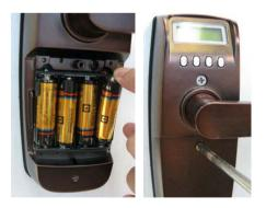
3) When batteries are inserted, two beeps are heard indicating that the lock is ready to program.
