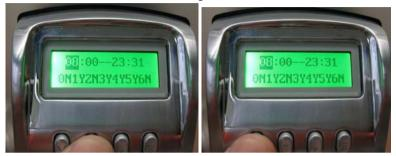
• Choose the correct "From" minute by using the Up/Down arrows until desired numeric minute is chosen and press "M" to save selection <u>OR</u> use the numeric keypad on the outside unit to enter the numeric minute and press "M" to save.
