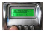
2) Use the up and down arrows to scroll thru the lock modes until the desired mode is reached and press "M" to save setting.
