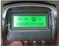
• Choose the correct "To" minute by using the Up/Down arrows until desired numeric minute is chosen and press "M" to save selection <u>OR</u> use the numeric keypad on the outside unit to enter the numeric minute and press "M" to save and go onto the **Days of the Week** set up.
