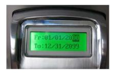
6) Use the up and down arrows (or numeric keypad on outside unit) to choose the appropriate MM, DD and YYYY in each section. When desired numeric value is chosen for each section, press "M" to move onto the next date value.
