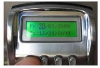
• Use the up and down arrows (or numeric keypad on the outside unit) to enter "15" (for the fifteenth day of the month) and press "M".
