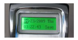
5) Choose the correct month by using the Up/Down arrows until desired numeric month is chosen and press "M" to save selection **OR** use the numeric keypad on the outside unit to enter the numeric month and press "M" to save.
