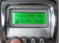
10) Choose the correct minute by using the Up/Down arrows until desired numeric minute is chosen and press "M" to save selection <u>OR</u> use the numeric keypad on the outside unit to enter the numeric minute and press "M" to save.
