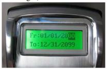
Use the up and down arrows (or numeric keypad on outside unit) to choose the appropriate MM, DD and YYYY in each section. When desired numeric value is chosen for each section, press "M" to move onto the next date value.
