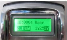
7) To **Delete FINGERPRINTS** associated to the specific User ID, scroll down to and highlight section **2.2 Del** and press "M".
