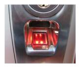
3) After the fingerprint sensor powers on, rest an enrolled fingerprint on the sensor window to verify.
