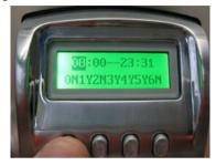
Choose the correct "From" minute by using the Up/Down arrows until desired numeric minute is chosen and press "M" to save selection <u>OR</u> use the numeric keypad on the outside unit to enter the numeric minute and press "M" to save.
