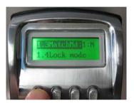
2) Use the up and down arrows to scroll thru the matching modes until the desired mode is reached and press "M" to save setting.
