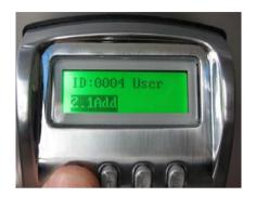
If no fingerprints have been enrolled for this User ID, then **1N**, **2N**, **3N** will be displayed. A total of 3 fingerprints (from fingers or thumbs) can be enrolled for each User ID. If there are fingerprints already enrolled for the User ID, then "Y" will be displayed next to some or all of the numbers.
