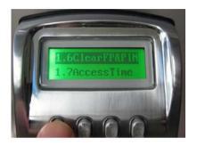
2) To delete all fingerprints, highlight the **Fingerprints** option and press "M".
