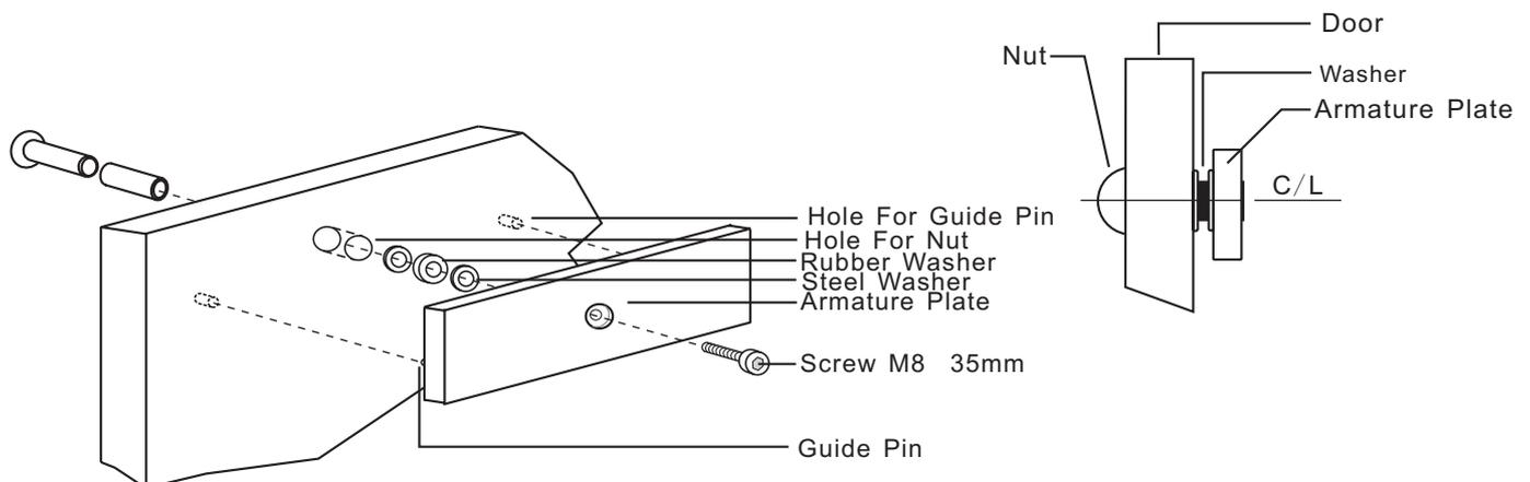
**\*\*Important:** Fix the armature plate not too tightly, and make the rubber washer more flexible, in order to make the armature plate automatically adjust its proper position with the magnet.
