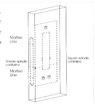
2. Drill the door from both sides with electric drill. Cut out the cavity for mortise as per drilling view in the manual.
