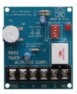
Model 6062 programmable timer is suitable for many functions that require a timed operation e.g. Access Control Applications, Siren/Bell Cut Off Module, Dialer Delay, Guard Tour Supervisory Timer, etc. Some optional functions include: One Shot, Delayed Release, Delayed Operate, Delayed Pulse and Pulser/Flasher.
